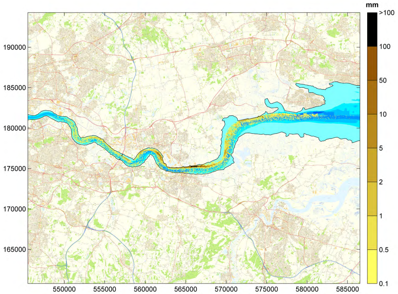
Figure 4.32: Maximum deposition depth of the released sediment during 5 days of dredging – Scenario 3 Background image contains OS data © Crown copyright (2016)
