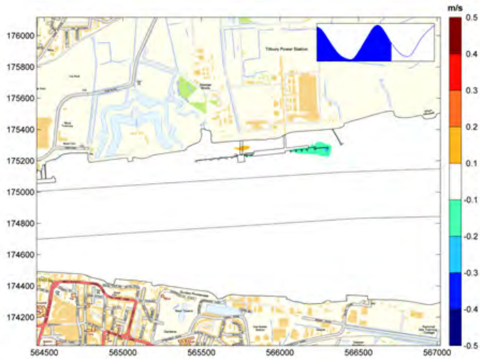
Figure 2.18: Difference in depth averaged current speed magnitude - proposed works compared to baseline, peak ebb tide
