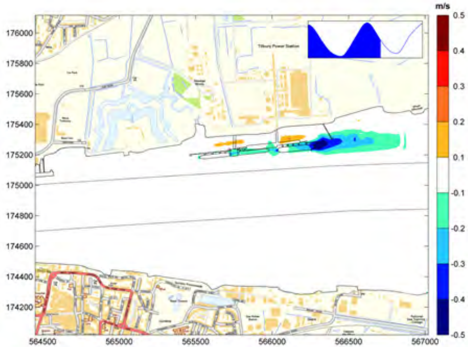
Figure 2.26: Difference in depth-averaged peak current speed magnitude - proposed works and vessels compared to baseline (no vessels), peak ebb tide
