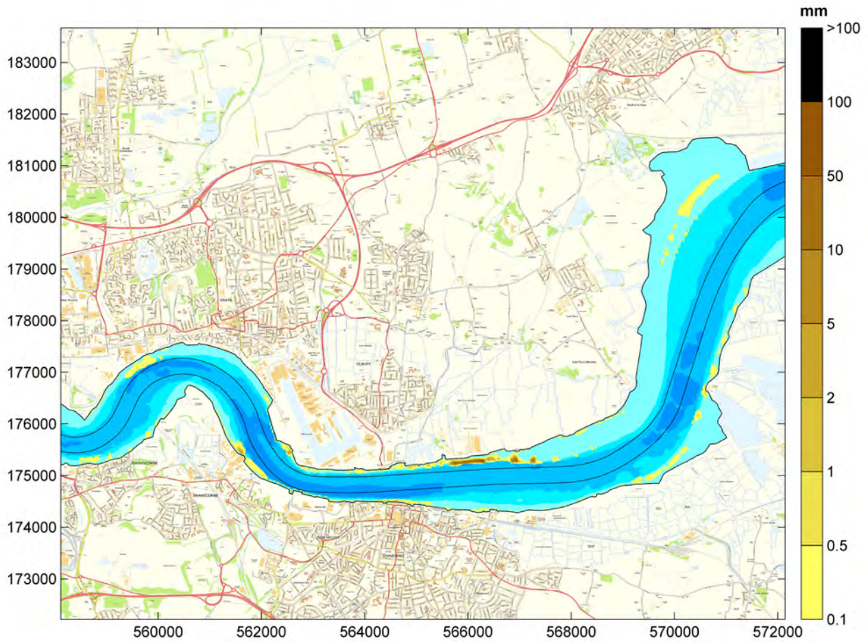
Figure 4.9: Nett accumulation of the released sediment at the end of 14 days of backhoe dredging Background image contains OS data © Crown copyright (2016)
