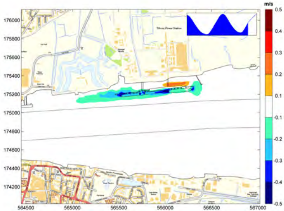
Figure 2.27: Difference in depth-averaged peak current speed magnitude - proposed works and vessels compared to baseline (no vessels), peak flood tide
