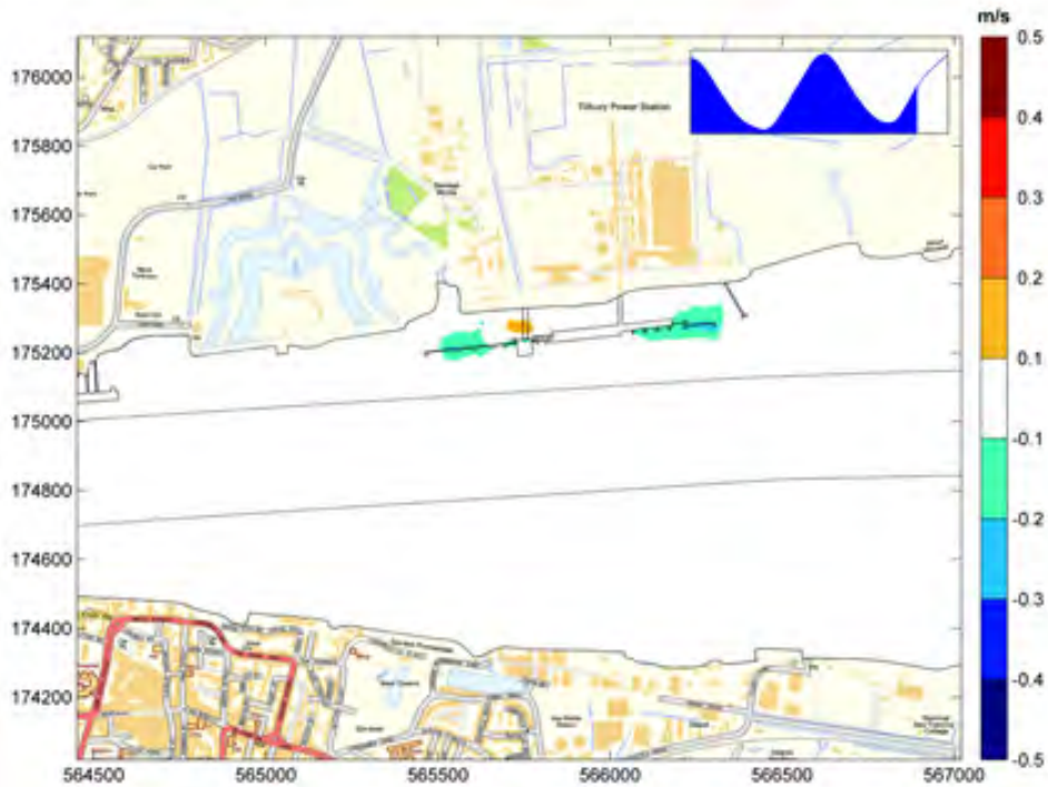
Figure 2.23: Difference in current speed magnitude - proposed works compared to baseline, near surface, peak flood tide
