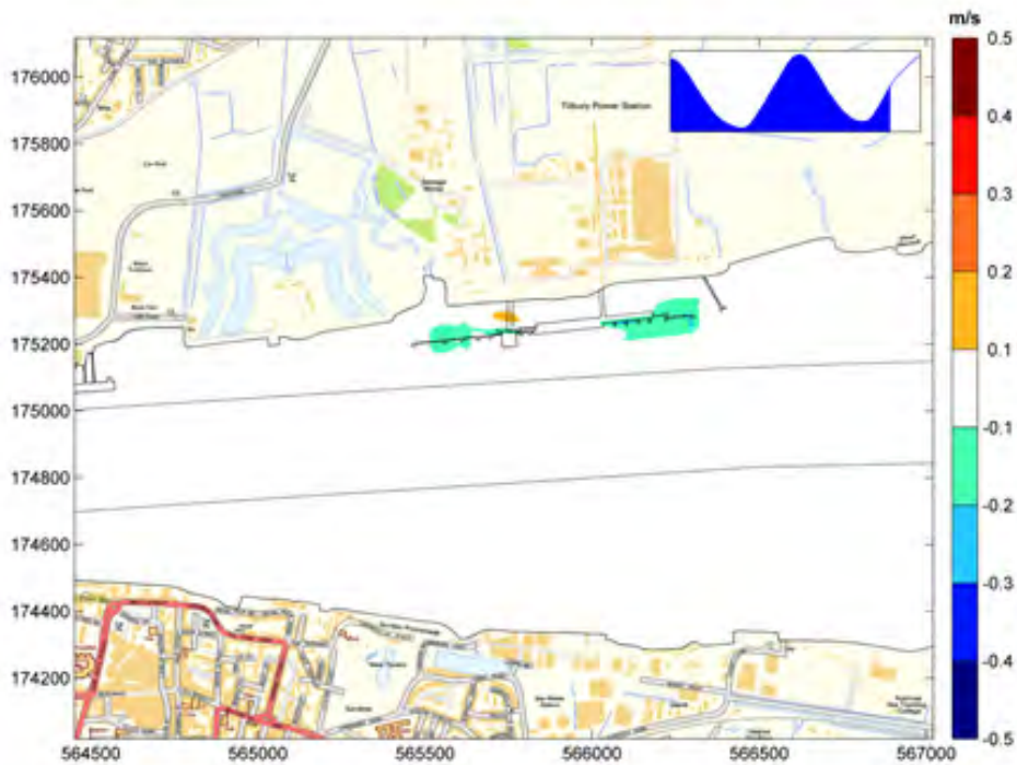
Figure 2.21: Difference in current speed magnitude - proposed works compared to baseline, near bed, peak flood tide
